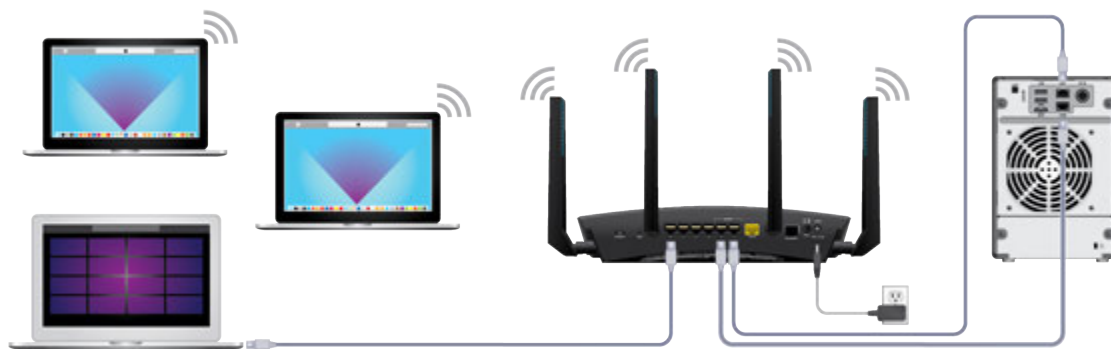
Figure 5. Ethernet port aggregation
