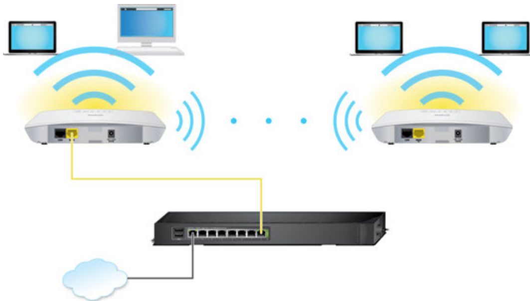
Figure 8. WiFi bridge configuration between two access points
